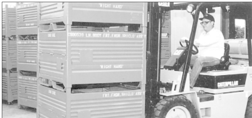
Corrugated steel stacking pallet boxes are perfect for sub-assemblies and inter-plant transport. Size and interior design are variable to meet your needs.
