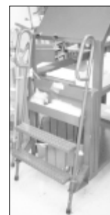
Detail of modified ladder truck showing optional paperwork tray and added front bin
