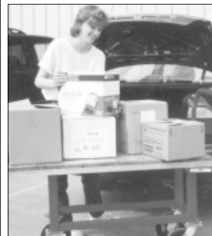
Elevated platform reduces loading effort, avoids injury.
