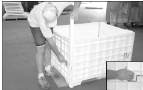
With all sides attached to the base, pull back on the extrusion lock. Remove the extrusion from one side and re-insert the extrusion so both sides are now connected. Continue this process around the bin and the assembly process is complete.
