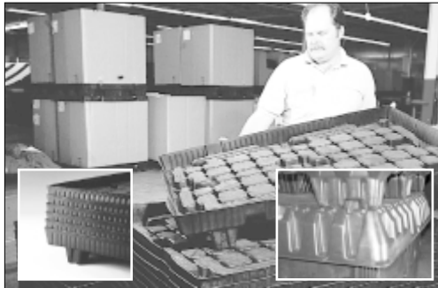
Mirror Image Interchangeable Pallets Provide Secure Interlocking Legs and Nestability
